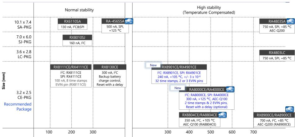
Backup Current Consumption.(nA Typ.): Current consumption value when RTC module is individually in operation, whereas the system's main MCU is on sleep mode
