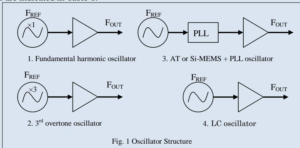
Fig. 1 Oscillator Structure
