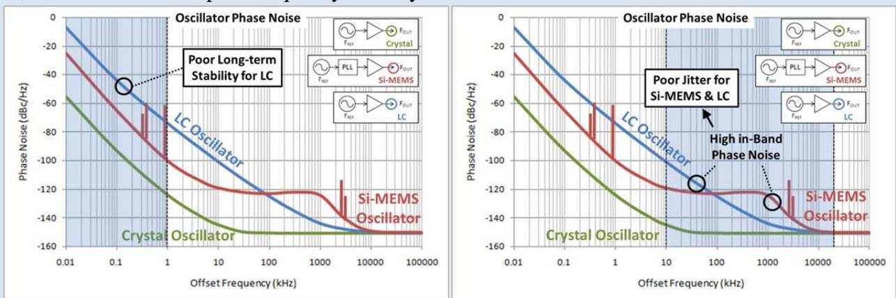
Fig. 6 Comparison of Carrier Vicinity (Low Band Side) Properties (left) and Floor Level (High Band Side) Properties (right)
