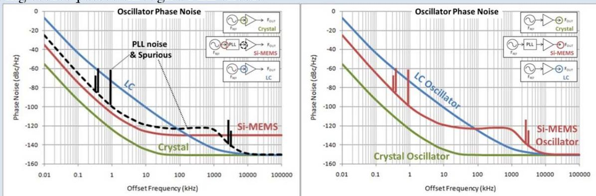
Fig. 5 PLL Circuit Phase Noise Property Image (left) and Phase Noise Property Tendencies based on Oscillator Structural Differences (right)
