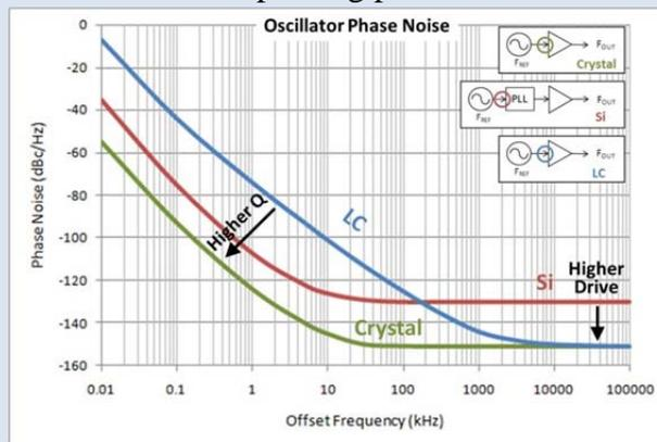
Fig. 4 Phase Noise Property Image of Oscillating Source
